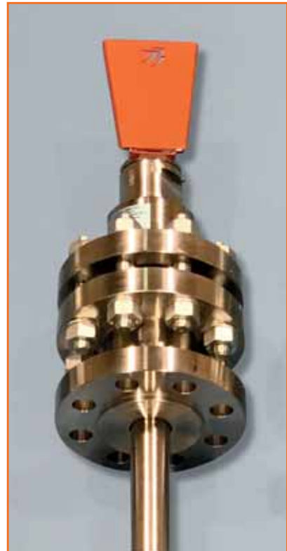
Intrusive Omni-Directional Pig Signaller 2" 600# Adjustable Pig Signaller with spool piece, wetted parts in 316L
